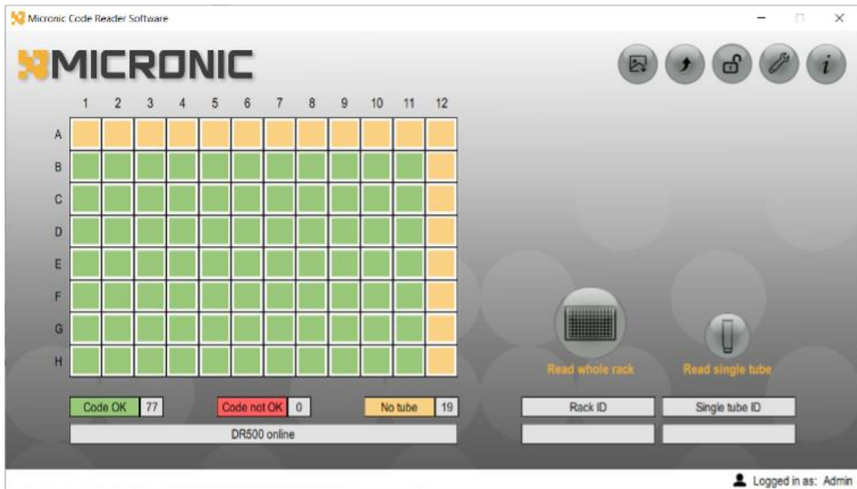
Fig 53: A Series of Cells in the Tube/Vial Decode Status Matrix as Yellow i.e. 'No Tube/Vial Detected'
