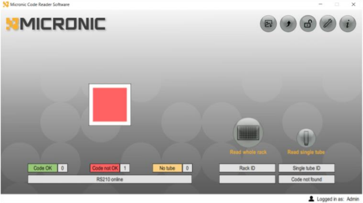
Fig 18: Review Result for Single Tube Code not OK/ No Tube
